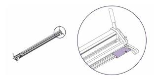
A material stop is mounted at both ends end of your SmartFold (seen highlighted in this image). When cutting tough or thick materials at prevents it sliding when being cut.
