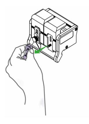
Pull the magnetic blade clamping plate away from the cutting head.
