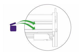
Put a small amount of petroleum jelly (Vaseline) on the scouring surface of a dish washing sponge and rub it up and down the two tracks. Wipe clean any surplus with a dry cloth.
