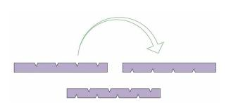
Both sides of the cutting strip can be used, it is important the strip is turned over in the correct orientation. The four tracks are offset to one side so when the strip is turned over correctly the new set of four tracks do not align with the originals.
