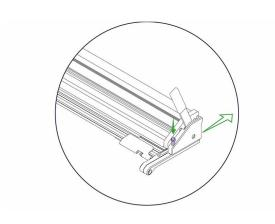
Press and hold down the highlighted button on the right side of the unit. Push the end of the cutter bar away from you.
