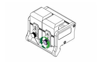
Undo the highlighted knob to remove the magnetic blade clamping plate.
