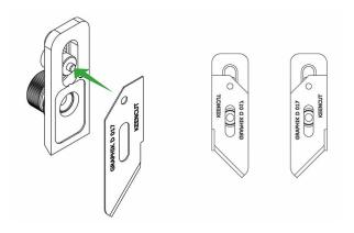
Insert a Graphik blade, check it is facing the correct way for your desired direction of cutting. Place the small pin in the hole at the top of the blade and align with the edge of the clamping plate.
