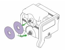
Choose the creasing wheel you would like to use and exchange it with the lower wheel. Replace both clamping knobs.
