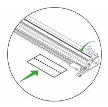
Pull the lever to raise the cutter bar, place the material for cutting approximately in position under the cutter bar.
