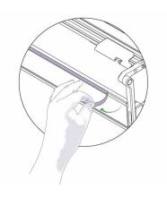
Remove the damaged sightline strip making sure that all residue from the adhesive tape is removed.
