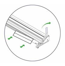
Push the lever to lower the cutter bar so it is only 1-2mm (1/16") above the surface of the material, the closer to the material it is the less lining up error you will get when viewing the cut marks.
