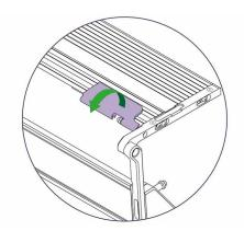
The material stop can be rotated to move it out of the way.
