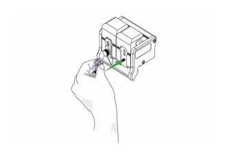
Replace the blade clamping plate onto the blade holder but do not tighten fully until the blade depth has been set (see how to adjust the blade depth >).
