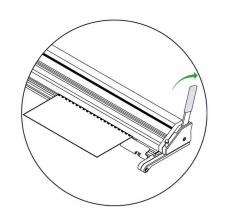
When fully aligned use the lever to lower the cutter bar onto the material and clamp it in position ready for cutting. Further cutting information is given in the sections under relevant tool heads.
