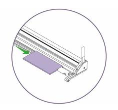
Position the board against the right hand material stop and clamp in place.
