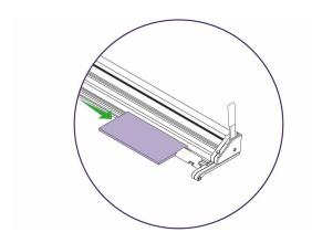
The material should be in contact with the material stop to prevent it moving when cutting.
