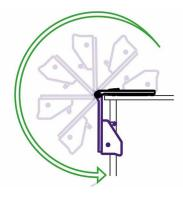
Grip the cutter bar firmly, lift carefully and swing over the edge of the bench, bring gently to a stop when vertical.
