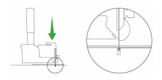
Check that the material is not being pushed into the cutting groove as the blade is cutting. If so, the material is likely to be suited to being cut with the rotary blade of the Fabric tool head where the underside of the material is supported on a plastic cutting strip. As a short term measure, it is possible to use the Graphik blade on the plastic cutting strip but too much use will quickly wear out the strip. Refer to the Fabric tool head for instruction to engage the cutting strip.
