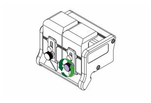
Undo the highlighted knob to remove the magnetic blade clamping plate.
