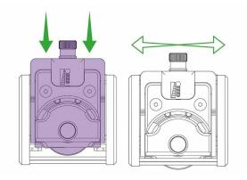
The Fabric tool head cuts in both directions and requires the blade holder to be pressed down fully whilst the rotary blade is cutting the material.
