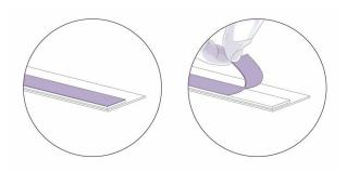
Your new sightline strip will have a protective backing on the double sided tape found on the underside of the part. Remove this backing.
