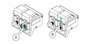
To adjust the height of the blade, loosen knob 'A' by a half to one full turn. Move knob 'B' up or down until the blade is long enough to just cut through the material.
