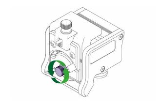
Loosen the clamping knob.
