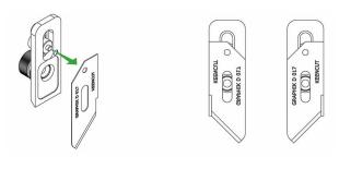
Lift off the blunt blade (if there is one) and replace with a new Graphik blade, check it is facing the correct way for your desired direction of cutting. Place the small pin in the hole at the top of the blade and align with the edge of the clamping plate.
