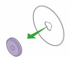
Separate the boss from the blade and inspect the boss for wear and clean off any debris. Dispose of the worn blade responsibly.
