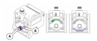
Rotate the red blade guard, using tab (B), to reveal or hide the blade. If it is difficult to rotate loosen the clamping knob (A) a little. Ensure it is adjusted correctly before cutting so the blade is just able to rotate without sideways movement.
