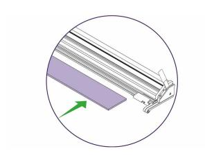
Insert your piece of material and lower the lift and hover so that it is just above the face of the material (as shown previously).
