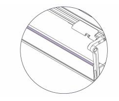
You will see the sightline strip on the underside of the cutter bar.
