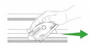
With the blade engaged, pull the Rocker tool head in one continuous motion along the material to achieve the best results.
