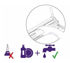
Moisten a cloth with diluted detergent to wipe down the cutter bar and base plate, dry with a cloth.
