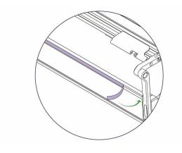
Apply the sightline strip in stages from left to right, ensuring that no wrinkles or bubbles form under the tape.
