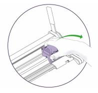
Gently lift to remove the cutter head, then replace end stop.
