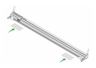
When cutting a small piece of board place it at one end of the cutter and place a scrap piece at the other end to keep the cutter bar parallel to the base.
