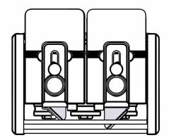
The blades also have adjustable cutting depth, so if a thick material is being cut on a long machine such that it is beneficial to make two cuts, one blade can be set to cut half the thickness in one direction and the other to cut full depth on the return journey.
