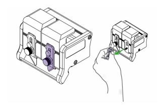
Pull the magnetic blade clamping plate away from the cutting head.
