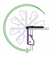
To change the sightline strip, first grip the cutter bar firmly, lift carefully and swing over the edge of the bench, bring gently to a stop when vertical.
