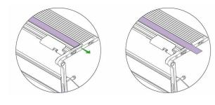
The cutting strip is removed by sliding it to the right, to keep the orientation of the strip correct the left hand end should remain on the left once turned over.
