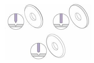
The three creasing wheels supplied with the Creaser tool head will each produce a different style of crease. Experiment on small samples of your material to see which gives best results.
