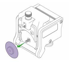
Remove the blade and magnetic blade boss. There may be a number of clear plastic shims on the threaded shaft, ensure they are clean and in good condition.
