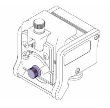
Check the blade is rotating and not moving from side to side, if it is, adjust the blade clamping knob.
