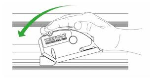
When cutting thinner / less dense materials, ensure the blade depth is adjusted so only the tip of the blade is going through the material. Place your hand on the Rocker tool head as shown and rock it forward to engage the blade.
