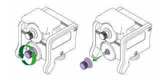
Remove the lower clamping knob.
