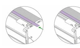
Turn over and re-insert the cutting strip so that the smooth surface is now facing upwards and what was the left hand end goes in first. Push it in nearly all the way, again use a flat edge under the left hand end to raise the strip above the adhesive patch, when in position press the strip onto the patch to prevent it sliding.
