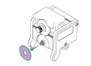
Remove the creasing wheel leaving the bearing and clear plastic shim in place.
