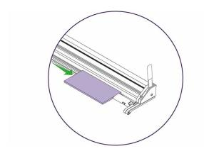
Butt the material up to the stop before clamping it in place.
