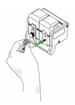
Replace the blade clamping plate onto the blade holder but do not tighten fully until the blade depth has been set. Repeat on the other blade holder if required.
