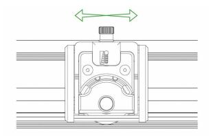
Cut in one smooth continuous motion, adjust to increase or decrease the cutting pressure if necessary.
