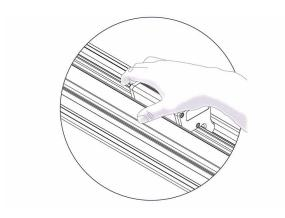
Position the cutting head to start the cut, turn your body to face to the right and place the palm of your right hand on the cutting head.
