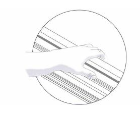
Extra effort can be applied by holding the grip area on the top of the cutter bar with your other hand and using the strength across your shoulders to push. Thicker materials can be cut in several passes.
