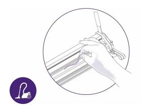
Use a vacuum cleaner to remove any dust and smaller debris. Frequency: daily as required
