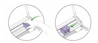
Insert the cutting head of your choice, and slide it to the left. More than one tool can be mounted on the cutter bar if required.
