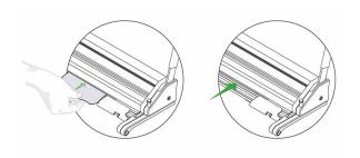
Place a piece of the material under the cutter bar so it does not protrude past the edge of the cutter bar and the blade can be seen against the edge of the material.
