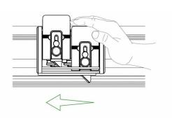
Depress the blade holder and push the cutting head using the strength across your shoulders.
